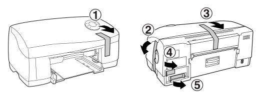
2 Open the front cover, and remove the protective material 6 shown in the illustration.
